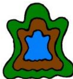
1205 Figure 7 Area yield of grain leather and split leather (green - raw hide, brown - grain leather, blue - split leather)
