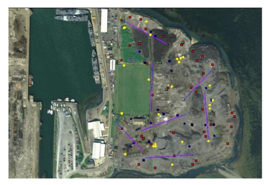
Fig. 3. Site investigation coverage: location of boreholes, trial pits, slit trenches and geophysics lines.
