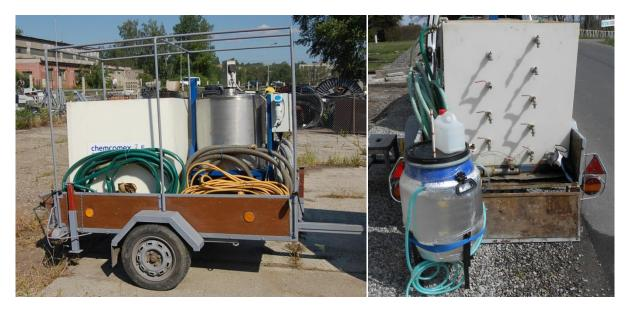
Fig. 1. Mobile system of IRON Technology (left) and its anaerobic reactor (right)
