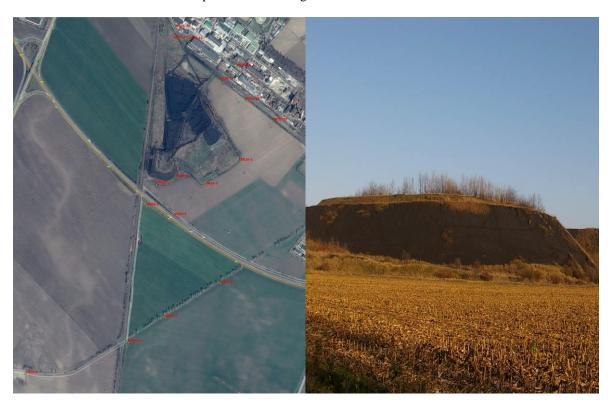
Fig. 1. Ground water monitoring net (red labels) in the surrounding of leach residue pile; southeastern view at the denuded part of leach residue pile (on the right)
