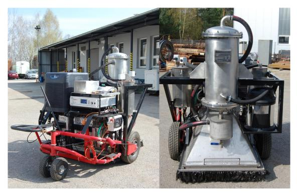
Fig. 2.VLNOCHOD Microwave remediation device
