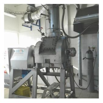
Fig. 2.Mixed dryer of semi-pilot testing unit.
