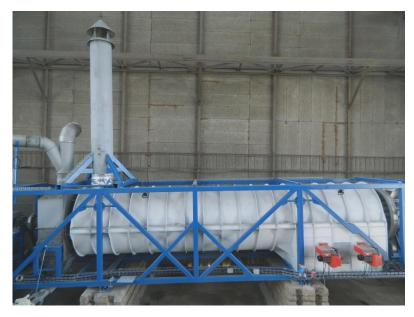
Fig. 4. Rotary kiln of continuous thermal desorption pilot unit.
