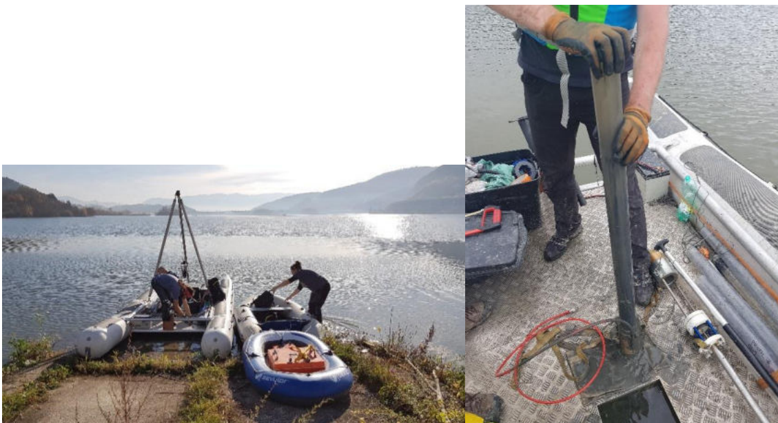
Fig. 1 Floating drilling platform and taking the drill core from the bottom of the dam
