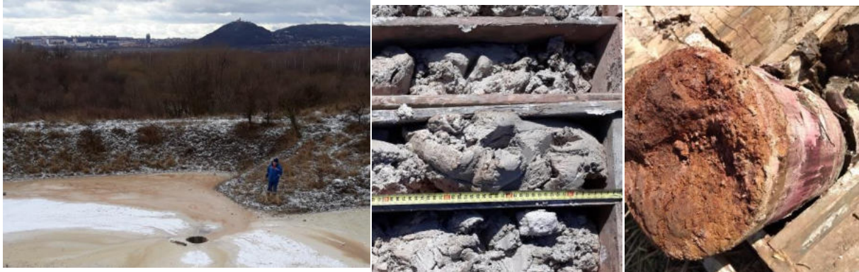
Fig. 2 Example of lime sludge dump (left), lime sludge consistency in drill core (center), and typical purple color of phenolic solution submerged tertiary clays in lime sludge underlying strata (right).
